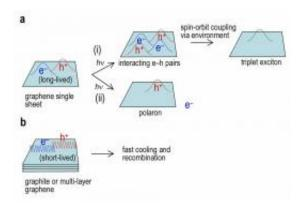
The new optical-induced absorption mechanisms [a] Photoexcitation of a dispersed graphene single sheet gives long-lived electron-hole pairs. Further excitation causes the appearance of localized states such as (i) excitons (neutral excited state) or (ii) polarons (charged excited state) due to interactions. [b] For comparison, graphite gives on electron-hole gas that is very short-lived due to fast cooling and re-combination. Credit: National University of Singapore
