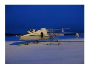
The Geophysica research aircraft serves as a platform to bring the GLORIA measurement instrument up to 20 kilometers height. Credit: Photo: Tobias Guggenmoser/FZJ
