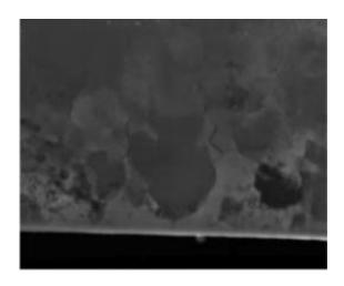
Iron, carbon, and oxygen subjected to intense temperatures and pressures form a pocket of iron oxide (bottom, center) and a darker pocket of diamond (bottom, right). Electron micrograph courtesy of Ohio State University.
