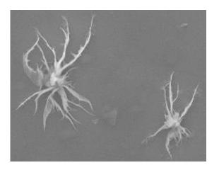
Microscopic, star-shaped flakes of functionalized graphene oxide plug holes in pores in a test of the material's ability to serve as a filter cake in fluids used to drill oil wells. The single-atom-thick flakes of treated carbon are pliable but among the strongest materials known. (Credit Tour Group/Rice University)
