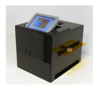
The millimeter-wave sensor can look through all non-transparent, non-metallic materials. Credit: Fraunhofer FHR
