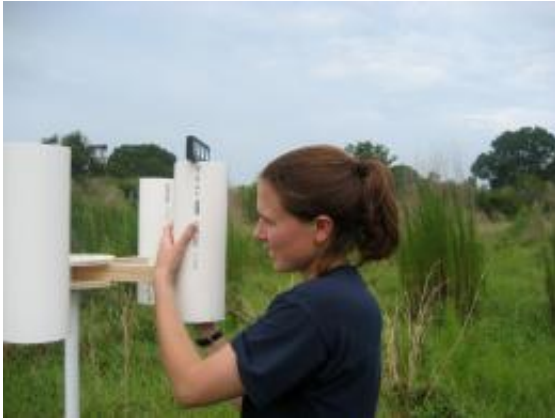
Laura Sherman setting up a sampling tripod to collect precipitation at one of the study sites near Crystal River, Florida. Credit: Emily White
