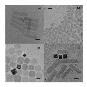
Transmission electron microscope images of CdSe colloidal nanoplatelets. Different lateral shapes (a-d) can be obtained using different precursors. Scale bars: b) 20nm, others, 10nm. Credit: Benoit Dubertret
