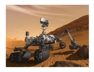
This artist concept features NASA's Mars Science Laboratory Curiosity rover, a mobile robot for investigating Mars' past or present ability to sustain microbial life. Credit: NASA/JPL-Caltech
