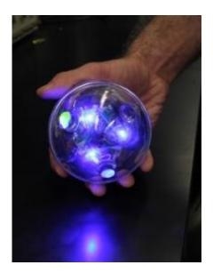
In the laboratory, a Sensorbot flashes out its code. By means of these brilliant blue pulses of light, the spherical undersea robot relays information about its environment. The light code is captured by high-speed cameras, which record and transmit the data for later analysis. Photo by: The Biodesign Institute at Arizona State University
