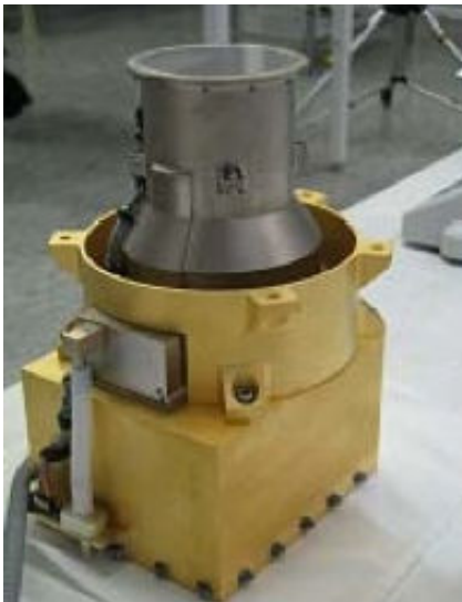
A photo of the Radiation Assessment Detector (RAD) in the laboratory
