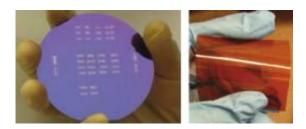
(Left) The fully printed back-gated SWCNT thin-film transistor printed on silicon dioxide. (Right) The fully printed top-gated SWCNT thin-film transistor printed on flexible Kapton. Image credit: Pochiang Chen, et al. ©2011 American Chemical Society
