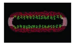
An illustrated cross-section of a nanotube UB chemists created. The green structures are negatively charged carboxylic acid groups, which help trap positively charged particles.
