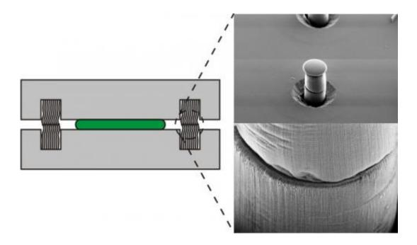
Two chips have interconnects that are filled with thousands of carbon nanotubes. The chips are then bonded with adhesive so that the carbon nanotubes are directly contacted. A connection using two such interconnects is pictured to the right. Credit: Teng Wang, et al. Carbon-Nanotube Through-Silicon Via Interconnects for Three-Dimensional Integration. Small, 2011, Volume 7, pages 2,313-2,317. Copyright Wiley-VCH Verlag GmbH & Co. KGaA. Reproduced with permission.
