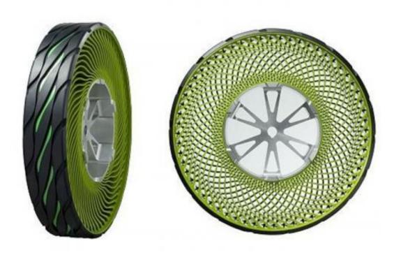
(PhysOrg.com) -- Visitors to the 42nd Tokyo Motor Show are to witness a new breed of airless tires from Bridgestone. Interest in the general press is already humming because of the material, design, and features of the Bridgestone debut on show. The concept tires use recycled thermoplastic, outside tread included. Fittingly colored green, the tires are being promoted for their green advantage of being completely
