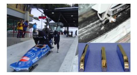
The friction levels of runners can now be measured accurately: top right, the measuring setup with runner and sensor in the ice channel; below right, various types of runner: (left to right) bob, skeleton and luge. Credit: Frauenhofer IWM
