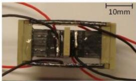
(Left) A diagram of the piezoelectric harvester with one straight inner piezoelectric multilayer stack (SIPMS) and two curved outer piezoelectric multilayer stacks (COPMSs). (Right) A photo of the first piezoelectric harvester prototype. Image credit: Tian Bing Xu, et al.
