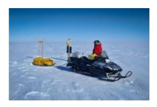
A corner cube reflector placed under the flight path of the AWI Polar-6 aircraft. The corner cube is used to validate the data from the ASIRAS instrument on Polar-6. Credits: UTAS-J. Beardsley
