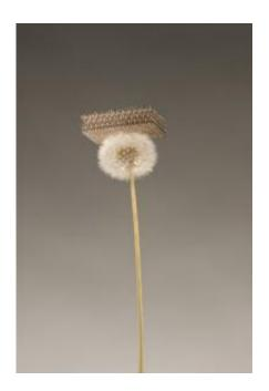
Ultralight metallic microlattice with a density of 0.9 mg/cm3. Image: HRL Laboratories, Photo by Dan Little
