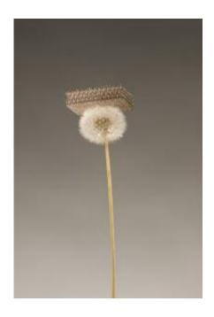
Ultralight metallic microlattice with a density of 0.9 mg/cm3. Image: HRL Laboratories, Photo by Dan Little
