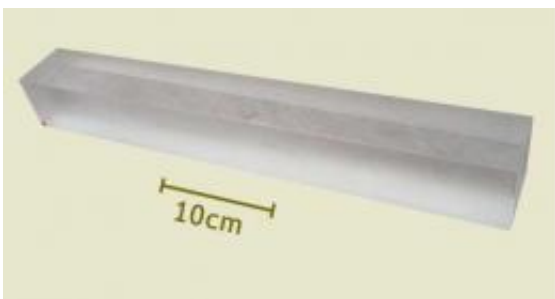
Figure 2: Light-collecting mirror prepared for the SPring-8 Angstrom Compact Free Electron Laser (SACLA) at the RIKEN Harima Institute. Credit: RIKEN
