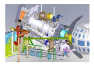
This is a design drawing showing bus-sized beam injector tilted upward relative to the DIII-D tokamak chamber on the left. Credit: Richard J. Buttery and M.R. Wade, General Atomics
