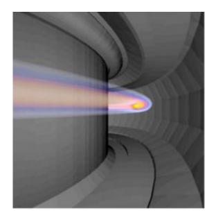
A computer-generated 3-D view shows runaway electrons in DIII-D based on high speed 2-D images of synchrotron emission from electrons traveling near the speed of light inside the tokamak. Credit: N.W. Eidietis and M.R. Wade, General Atomics
