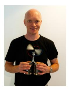
Ole Martin Løvvik demonstrates thermoelectricity with one glass of cold and one glass of hot water. The new technology utilises the temperature difference and generates enough energy to operate a rapidly rotating fan. Foto: Yngve Vogt
