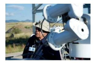
John Hickey, who developed the cavity for the first radiometer that went up in space, stands next to two automatic Hickey-Frieden Absolute Cavity Radiometers at the annual radiometer calibration event at NREL. Credit: Dennis Schroeder
