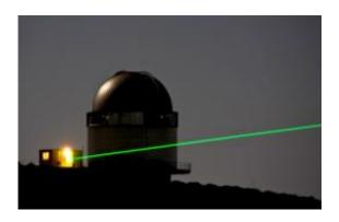
The Observatorio del Roque de los Muchachos on the island of La Palma housed the equipment to transmit the infrared signal and green guidance laser across the Atlantic Ocean to the receiving station in Tenerife. The experiment was carried out to test a new satellite mission concept for measuring concentrations of atmospheric carbon dioxide and methane. Credits: ESA
