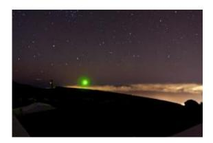
A green laser was used to guide the invisible infrared beam from La Palma to Tenerife as part of an experiment to test a new satellite concept for measuring atmospheric greenhouse gases and turbulence. Credits: ESA
