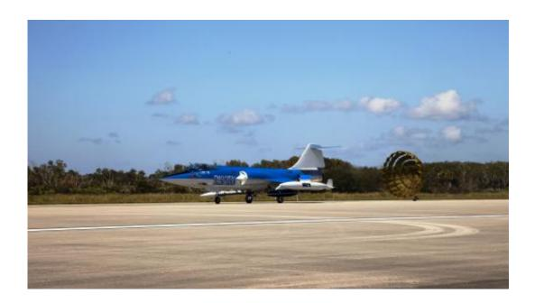
On Oct. 27th, the Star Lab launcher was tested out while attached to the F-104 carrier aircraft via a series of fast-taxis up and down NASA's Shuttle Landing Facility located in Florida. Credit: NASA.gov
