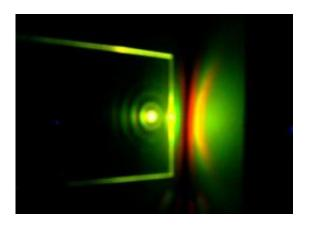
An LSC is illuminated by a laser beam (central spot) resulting in luminescence that is emitted from the edges and projected onto a white business card. The faintly visible concentric rings and different colors of light on the business card result from microcavity effects. Credit: Chris Giebink, Penn State
