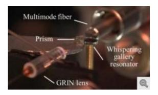
In the setup for this experiment, a telecommunication-compatible infrared beam is coupled to the whispering-gallery resonator through a diamond prism and the generated near-infrared, visible, and ultraviolet light are collected by a multimode fiber. Credit: Photo courtesy of Mona Jarrahi
