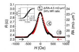
Resistance vs magnetic field of the Co2Fe(Al0.5Si0.5) (4 nm)/Ag(2 nm)/Co2Fe(Al0.5Si0.5) (4 nm) trilayer CPP-GMR device measured at room temperature and the schematic "scissors-type" magnetization configuration of the two Co2Fe(Al0.5Si0.5) free layers. Inset is the magnetization curve of the unpatterned trilayer film.
