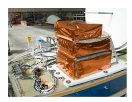
NASA Goddard's Cloud Physics Lidar electronics are installed in the upper area of NASA's Global Hawk unmanned aircraft just in front of the aircraft's communications antenna. Credit: NASA / Tom Tschida
