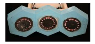
Based on simulations, the researchers have developed a manufacturing technique that can combine multiple modules as shown above. Here, three modules are mounted on a base of silicon rubber. The overall unit bends freely, so it can conform and adhere tightly to a curved surface such as the outside of a pipe. Despite their proximity, the three modules operate independently with no interference.
