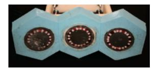
Based on simulations, the researchers have developed a manufacturing technique that can combine multiple modules as shown above. Here, three modules are mounted on a base of silicon rubber. The overall unit bends freely, so it can conform and adhere tightly to a curved surface such as the outside of a pipe. Despite their proximity, the three modules operate independently with no interference.
