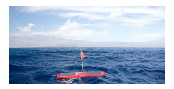
On the above-water part of the Wave Glider, solar cells recharge a battery that powers data sensors and transmitters. Underwater fins use wave energy for propulsion. Image credit: Liquid Robotics
