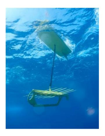
The self-propelled Wave Gliders use wave energy for propulsion. Image credit: Liquid Robotics
