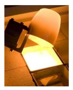
A robot arm takes over the fully automatic handling of the test melts in the glass screening unit - here, the pouring of the melt into the sample form. Credit: Knud Dobberke for Fraunhofer ISC
