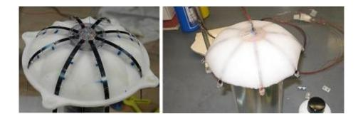
Engineers at Virginia Polytechnic Institute and State University (VirginiaTech) have developed a robot that mimics the graceful motions of jellyfish so precisely that it has been named Robojelly. Developed for the Office of Naval Research in 2009, this vehicle was designed to conduct ocean underwater surveillance, enabling it potentially to detect chemical spills, monitor the presence of ships and submarines, and observe the migration of schools of fish.
