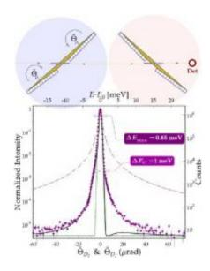
Experimental scheme and combined spectral resolution function of the blue-winged CDFDW monochromator measured against the red-winged CDFDW analyzer. The purple circles show spectral resolution function, the black solid line - spectral functions calculated using multi- crystal dynamical theory of x-ray diffraction. Other functions with the same bandwidth are shown for comparison: green dashed line - Gaussian; dark-red dash-dotted line - Lorentzian.
