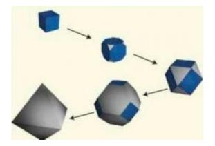
Schematic representation of polyhedral shapes accessible using the silver polyol synthesis developed by Peidong Yang, et. al. Credit: Image courtesy of Berkeley Lab
