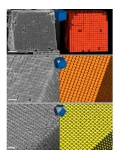
On the left are micrographs of supercrystals of silver polyderal nanocrystals and on the right the corresponding diagrams of their densest known packings for (from top-down) cubes, truncated cubes and cuboctahedra. Credit: Image courtesy of Berkeley Lab
