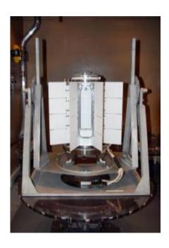
The Mars Science Laboratory's radioisotope power system was fueled and tested at Idaho National Laboratory. Here, magnetic testing ensures that the electric field generated by the system is small enough that it won't interfere with the rover's scientific instruments. Credit: Idaho National Laboratory
