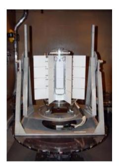
The Mars Science Laboratory's radioisotope power system was fueled and tested at Idaho National Laboratory. Here, magnetic testing ensures that the electric field generated by the system is small enough that it won't interfere with the rover's scientific instruments. Credit: Idaho National Laboratory
