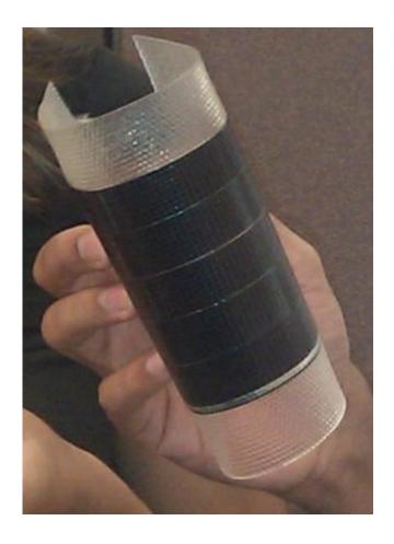
Thin film solar cells fabricated from gallium arsenide have achieved a record sunlight-to-electricity conversion efficiency of 28.4 percent. (Image courtesy of Alta Devices, Inc.)
