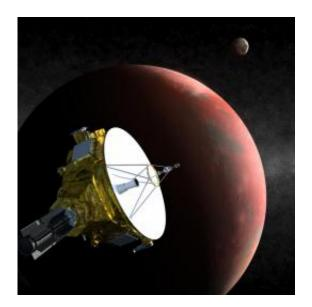
An artist's concept of the New Horizons spacecraft as it visits Pluto in 2015. Instruments will map Pluto and its moon, Charon, providing detail not only on the surface of the dwarf planet, but also about its shape, which could reveal whether or not an ocean lies beneath the ice. Credit: NASA/Johns Hopkins University Applied Physics Laboratory/Southwest Research Institute
