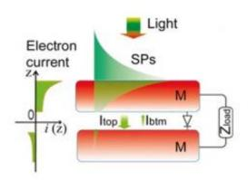
Surface plasmons on the top electrode in the MIM device can increase the current from the top electrode so that it is greater than the current from the bottom electrode, generating a positive net current. Image credit: Wang and Melosh. ©2011 American Chemical Society
