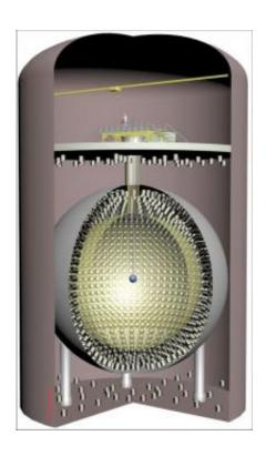
In the proposed test for a fourth neutrino, a small electron antineutrino source (blue) located at the center of a large liquid scintillator detector would be used to bombard a target. The red curve represents the oscillation of the antineutrino rate as a function of the distance within the detector. If the bombardment involves sterile neutrinos, interactions of the electron antineutrinos would show a spatial modulation of a few percent over a few meters. Image credit: L. Scola (CEA)
