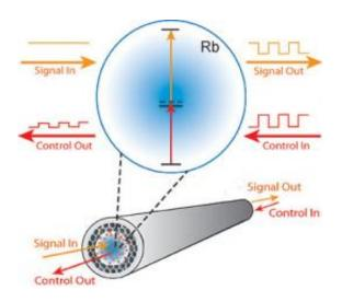
Rubidium atoms will absorb photons only if two photons of specific wavelengths arrive at the same time. This allows one stream of photons to turn another on or off. (Gaeta Group)
