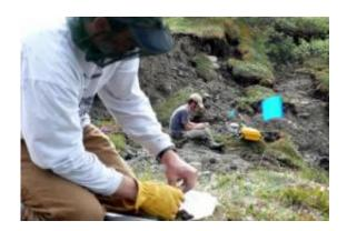
Ben Abbott, graduate student, right, and Jay Jones, professor of biology, both of the Institute of Arctic Biology at the University of Alaska Fairbanks collect soil cores and gas flux measurements from a landscape north of the IAB Toolik Field Station on the North Slope where permafrost has thawed and the ground has collapsed - called a thermokarst. Abbott and Jones are part of the National Science Foundation funded thermokarst project #08-0341. Credit: Photo by Marie Gilbert/IAB.
