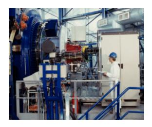
NAOS-CONICA installed at the 8.2 m telescope Yepun, which is part of the VLT. The dark blue ring on the left is the telescope adapter; the adaptive optics system NAOS is the adjacent light-blue part, and the camera CONICA is contained in the red cryostat. The white cabinet contains electronics used to control the instrument.
