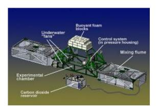
This diagram shows some of the main components of the deep-water FOCE system. The foam blocks are in different places on the current version of the experiment. Credit: © 2011 MBARI
