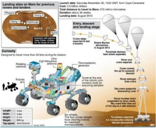
Graphic of the Mars Science Laboratory, an elite six-wheeled vehicle powered by nuclear fuel, is scheduled to launch at 10:02 am (1502 GMT) from Cape Canaveral Air Force Station in Florida atop an Atlas V rocket.
