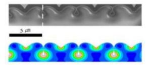
Researchers at Brown University and in Korea used focused ion beams to extract a cross-section of compressed gold nanofilm. When tips of regular, neighboring folds touched, nanopipes were created beneath the surface. Credit: Kyung-Suk Kim lab, Brown University
