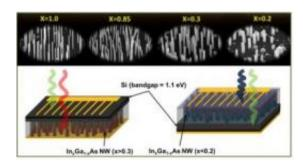
Solar cells (bottom) made with arrays of nanowires. Engineers can tune the performance by using nanowires of differing composition and thickness (top). Credit: Xiuling Li. University of Illinois
