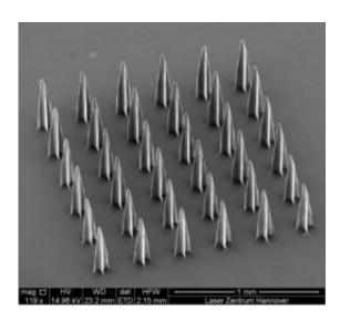
This array of microneedles was created, four needles at a time, by a four-beam two-photon polymerization system. The scale at the bottom shows a length of 1 millimeter. Credit: *Biomedical Optics Express*
