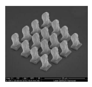
This image, taken by a scanning electron microscope, shows 16 micro-Venus structures that were produced simultaneously by a 16-beam two-photon polymerization system. The width of the entire array is less than the diameter of a typical human hair. The 16 structures were produced in approximately 45 seconds. Credit: *Biomedical Optics Express*
