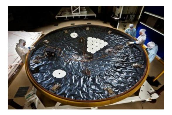
The MSL Entry, Descent and Landing Instrument (the black box in the middle left of the photo) is scheduled to launch as part of the Mars Science Laboratory mission. Credit: NASA
