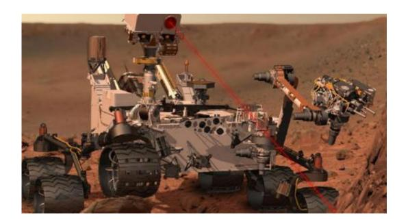
This artist's concept depicts the rover Curiosity, of NASA's Mars Science Laboratory mission, as it uses its Chemistry and Camera (ChemCam) instrument to investigate the composition of a rock surface. ChemCam fires laser pulses at a target and views the resulting spark with a telescope and spectrometers to identify chemical elements. The laser is actually in an invisible infrared wavelength, but is shown here as visible red light for purposes of illustration.
